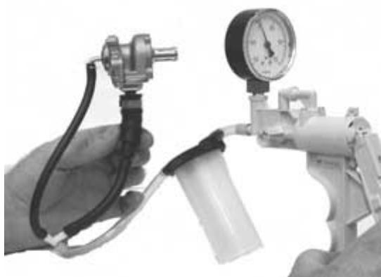
LA MANCANZA DI TENUTA DELLA VALVOLA CUT - OFF COMPORTA UNA RUMOROSITÀ ALLO SCARICO (SCOPPI IN MARMITTA). L'ERRATA TARATURA DELLA VALVOLA CUT - OFF PUÒ PREGIUDICARE LA CORRETTA FUNZIONALITÀ DEL CATALIZZATORE
